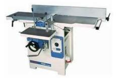
The FS 30 is a rigid and robust machine with a steel base and cast iron thicknesser worktables able to machine components of large dimensions guaranteeing maximum machining precision and the complete absence of vibration.
